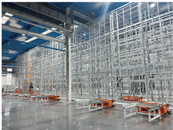
Three-Dimensional Raw Material Storage >>>
